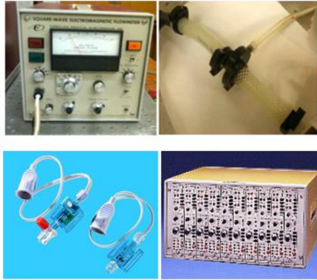
Figure 2.6: FM501 Electromagnetic flow meter (Upper left) and EP640 flow probe (Upper right); blood pressure transducers (lower left) and bridge amplifiers (lower right).
